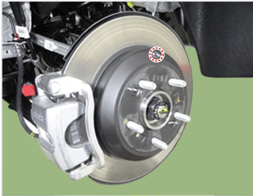
3. Rotate the toothed wheel of adjuster (A) by a screw driver until the disc is not moving, and then return it by 3 notches in the opposite direction.
